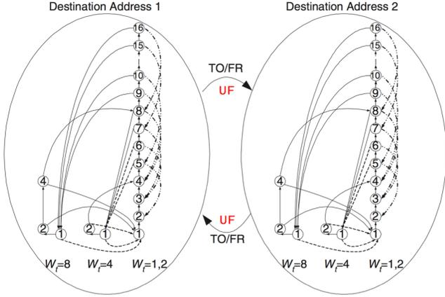
Fig. 1: SCTP Markov Chain state transition diagram with multi-homing. NOTE: UF events only in modified SCTP model.
