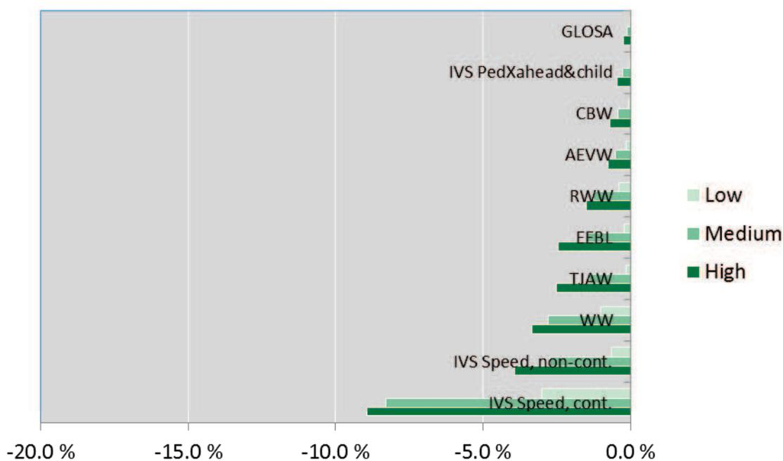
Figure 2: The overall safety impacts of cooperative functions in 2030 with vehicle penetration scenarios: low, medium and high
