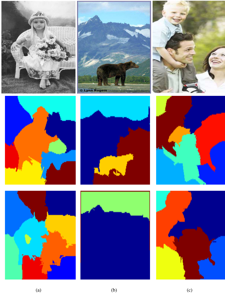
Figure 12: Another set of examples of image segmentation. The segmentation results using the proposed algorithm and Zelnik-Manor and Perona’s self-tuning spectral clustering algorithm are shown in the middle and bottom row respectively. From left to right, the optimal number of segments K_o were determined as 9,4,8 using our algorithm. They were estimated as 9,2,7 using the self-tuning approach.
