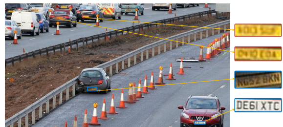
Fig. 1. Example illustration of vehicle license plates obtained by a video camera in the real scenario. The VLPs marked by red rectangle are in the extremely LR condition which are nearly unrecognizable. The VLPs marked by blue rectangle contain intact semantic information although it is unclear.
