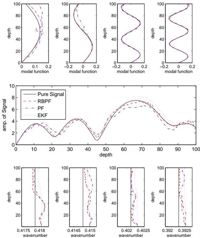
**Fig. 1.** Results of estimation and ground truth under SNR = 10 dB for: modes 1, 2, 4 and 5 (top), pressure field (middle) and corresponding wave numbers (bottom).
