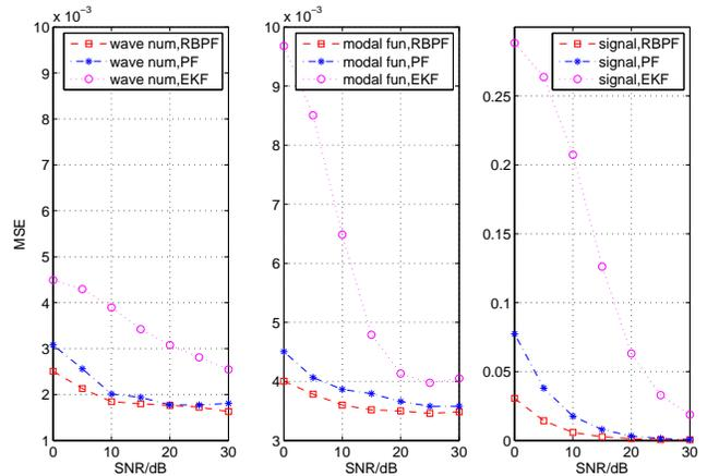
**Fig. 2.** RMSE versus different SNRs for wave numbers (left), modal functions (center) and signal field (right)
