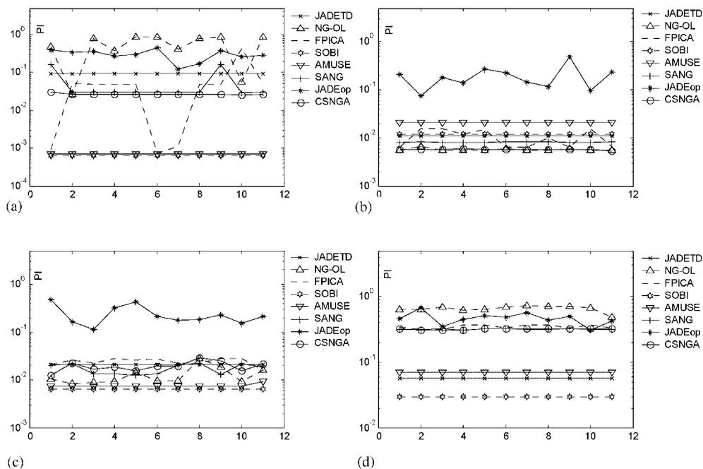
Figure 4. PI comparison of the proposed algorithm (CSNGA) with several other BSS algorithms (JADETD, NG-OL, FPICA, SOBI, AMUSE, SANG, JADEop) for the separation of four kinds of signals with cyclostationary properties. The four signals are, respectively, sinusoid signals, BPSK modelled signals, AR modelled signals and speech signals.
