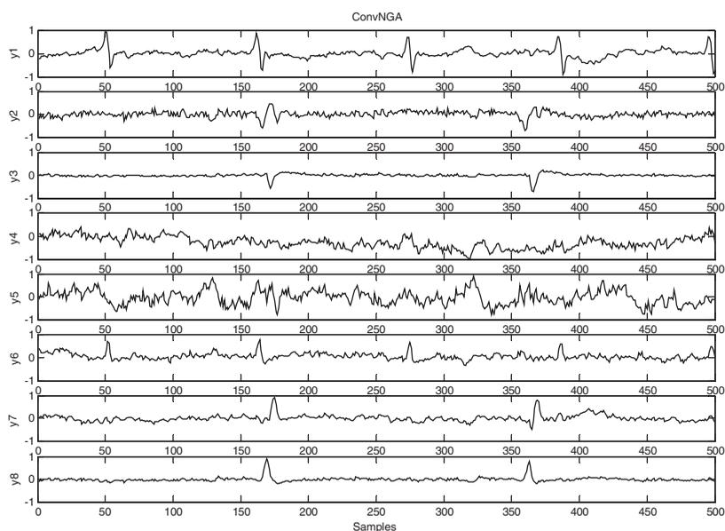
Figure 11. Separation results with ConvNGA algorithm for ECG signals in Figure 9.
