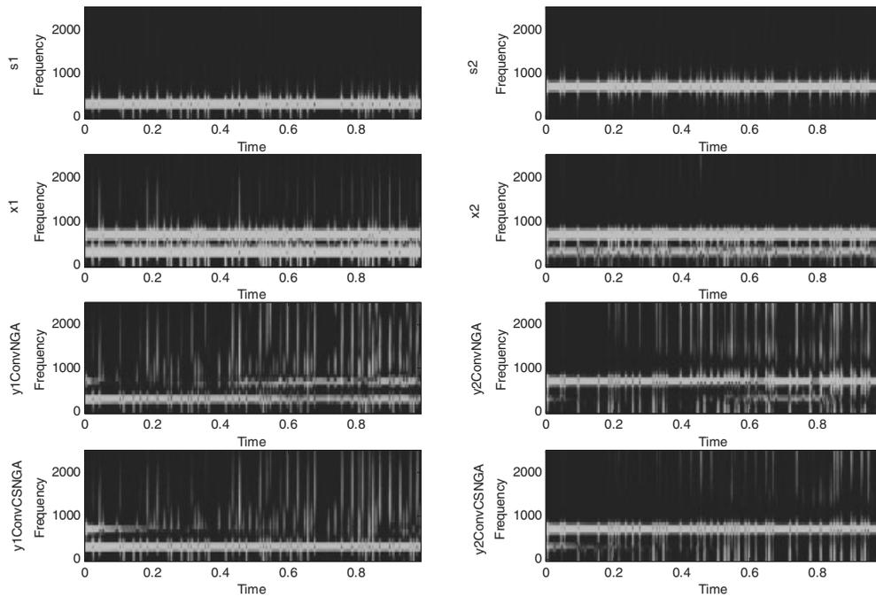
Figure 6. Separation of two BPSK source signals; the meanings of the symbols are identical to those in Figure 5.
