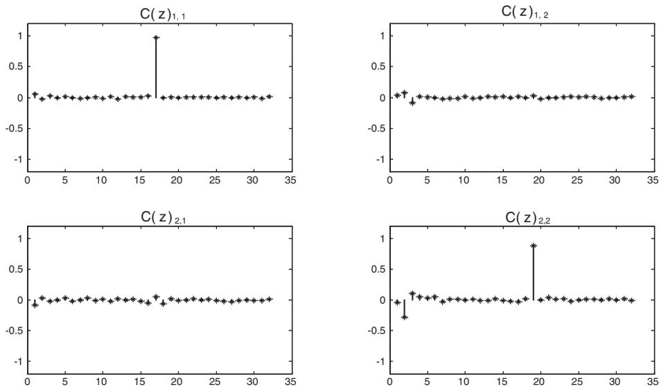
Figure 7. Simulation results of the global parameters of  $C(z)$  of the TITO system after convergence.
