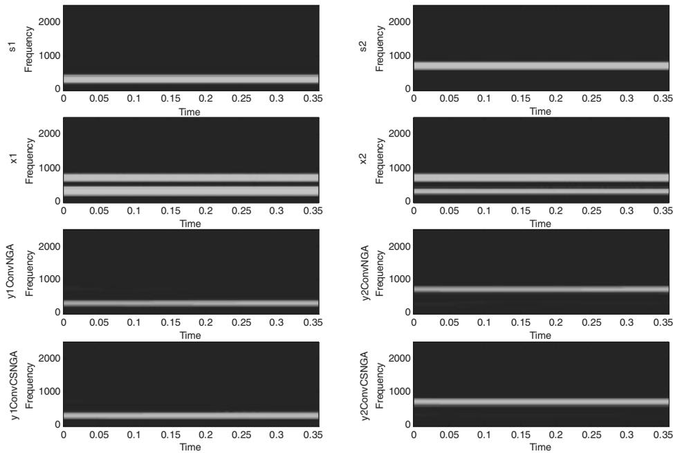
Figure 5. Separation of convolutive mixtures of two sinusoid signals:  $s_1$  and  $s_2$  are two sources,  $x_1$  and  $x_2$  are the two convolutive mixtures,  $y_1\text{ConvNGA}$  and  $y_2\text{ConvNGA}$  are the recovered signals by the natural gradient algorithm,  $y_1\text{ConvCSNGA}$  and  $y_2\text{ConvCSNGA}$  are the recovered signals by the proposed method.
