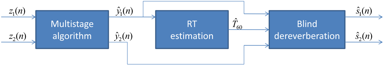
Figure 2: Block diagram showing the second scheme for the proposed joint blind dereverberation and separation algorithm. z_1(n) and z_2(n) are the available mixtures (microphone signals).
