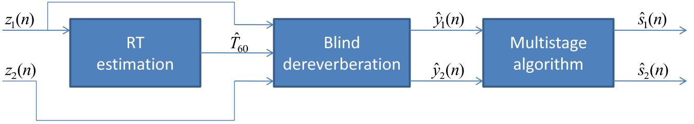
Figure 1: Block diagram showing the first scheme for the proposed joint blind dereverberation and separation algorithm. z_1(n) and z_2(n) are the available mixtures (microphone signals).
