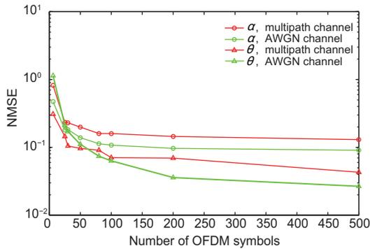
Fig. 5 The normalized mean-squared error (NMSE) of the estimated I/Q imbalance parameters versus the number of symbols ( $\alpha$ : gain imbalance;  $\theta$ : phase imbalance)
