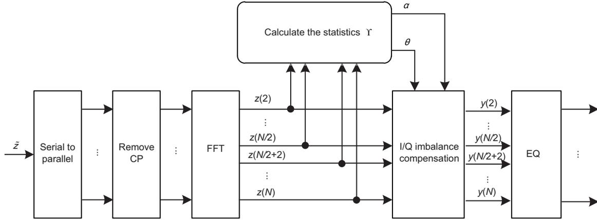
**Fig. 3** The framework of the proposed I/Q imbalance compensation scheme in OFDM direct-conversion transceivers (CP: cyclic prefix; EQ: equalization)
