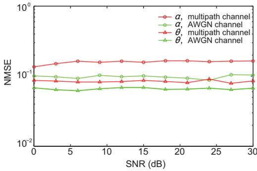
Fig. 4 The normalized mean-squared error (NMSE) of the estimated I/Q imbalance parameters versus the SNR of received signals ( $\alpha$ : gain imbalance;  $\theta$ : phase imbalance)
