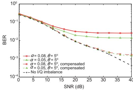
**Fig. 7** The bit error rate (BER) of the compensated received signal at different SNRs in the multipath channel with different gain imbalances ( $\alpha$ : gain imbalance;  $\theta$ : phase imbalance)
