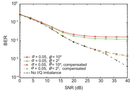
**Fig. 9** The bit error rate (BER) of the compensated received signal at different SNRs in the multipath channel with different phase imbalances ( $\alpha$ : gain imbalance;  $\theta$ : phase imbalance)
