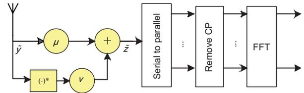
Fig. 2 Block diagram representation of an OFDM system with I/Q imbalances (CP: cyclic prefix)
