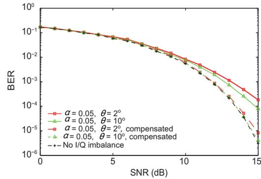
**Fig. 8** The bit error rate (BER) of the compensated received signal at different SNRs in the AWGN with different phase imbalances ( $\alpha$ : gain imbalance;  $\theta$ : phase imbalance)
