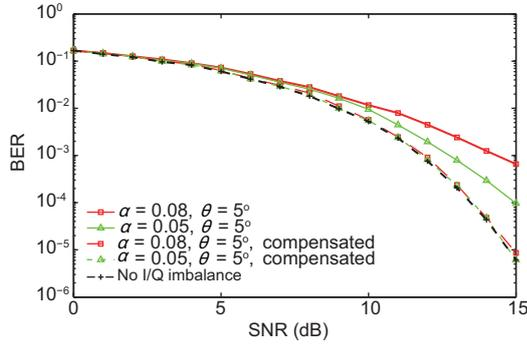
**Fig. 6** The bit error rate (BER) of the compensated received signal at different SNRs in the AWGN with different gain imbalances ( $\alpha$ : gain imbalance;  $\theta$ : phase imbalance)
