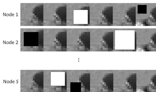
Fig. 3. Example of nodes in the spatio-temporal domain. The cuboid is flattened with respect to time to show subpatches at different temporal offsets.
