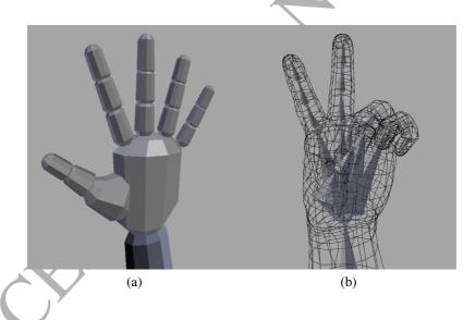
Figure 4: Kinematic hand model constructed in Maya. (a) The hand is broken into separate rigid bodies, joined through constraints to reflect realistic limitations. (b) The model is also rigged with a poseable skeleton allowing the generation of training data, and use in 3D applications.
