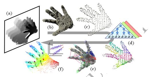
Figure 2: Method overview which shows processing of the depth camera stream (a). The depth is converted to its corresponding point cloud (b) for filtering and sub-sampling (c). Forest classification labels each point using depth (d), allowing constraint-driven model optimisation (e). Linear regression using depth sampled features then corrects model discrepancies(f).
