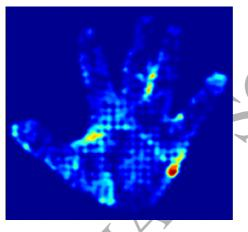
Figure 6: Residual constraint error from using a model with rigid components when converged using an ideal segmentation of depth. This error is synonymous with the use of a general hand model, and inter-person variation.
