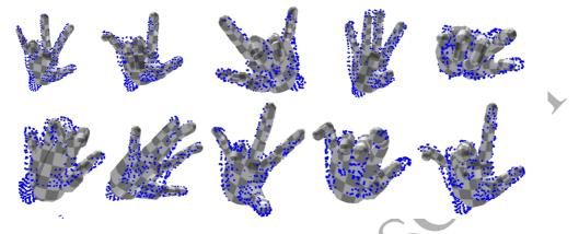
Figure 20: Qualitative Evaluation: examples of the combined descent method fitting to point cloud data. The kinematic model prevents self-intersection between fingers and provides realistic results.
