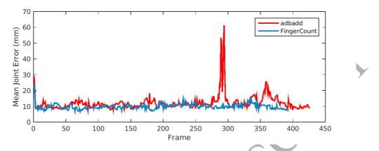
Figure 13: This graph presents the joint error for each frame for two sequences of the Dexter1 dataset. These two sequences illustrate the best and worst performance. A loss of tracking can be seen around frame 240 which is recovered from quickly due to the method being a hybrid approach, performing reinitialisation.
