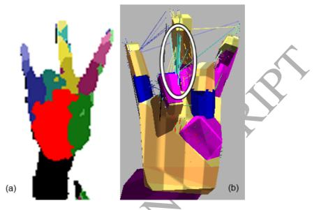
Figure 5: Constraint driven optimisation. (a) The hand's depth following segmentation of the Random Decision Forest. (b) The kinematic hand model after optimization using constraints. The ellipse highlights the finger being correctly estimated, despite erroneous constraints that are overpowered through optimisation.
