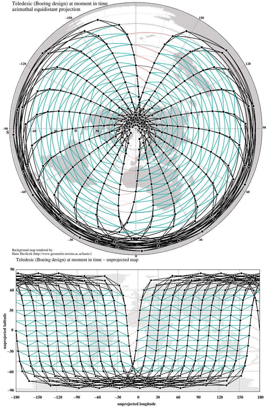
Figure 2-5. A star constellation: The 288-active-satellite Boeing *Teledesic* proposal
