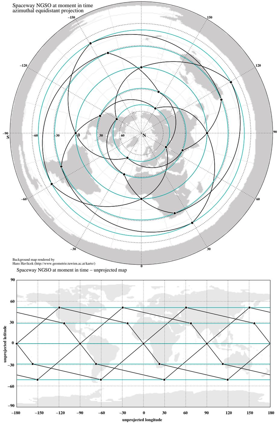
Figure 2-4. A rosette constellation: the 20-active-satellite Spaceway NGSO proposal
