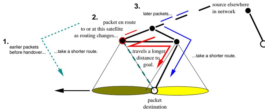
*Figure 2-7.* How handover can affect traffic in flight
