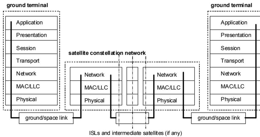
Figure 2-3. Full networking and routing approach, e.g. Iridium, Teledesic
