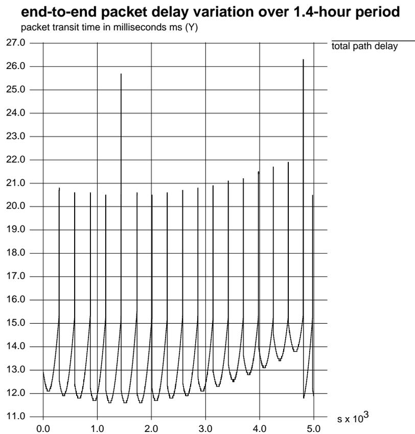
Figure 2-8. Path delay for high-rate traffic over a small timescale
