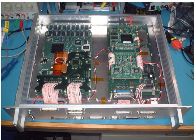
On left: SSTL SDR assembly. On right: router assembly.
