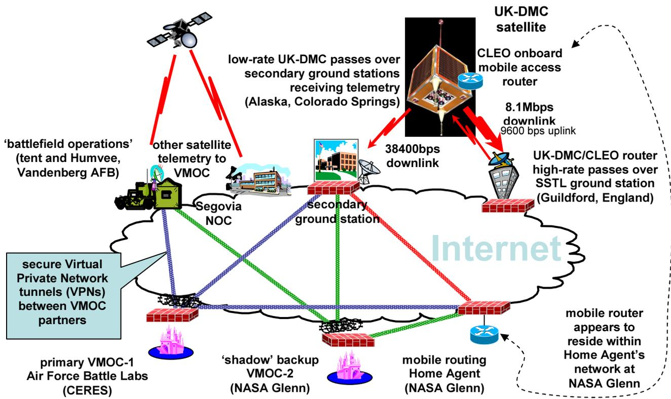
Figure 3. Network topology for the Vandenberg demonstration
