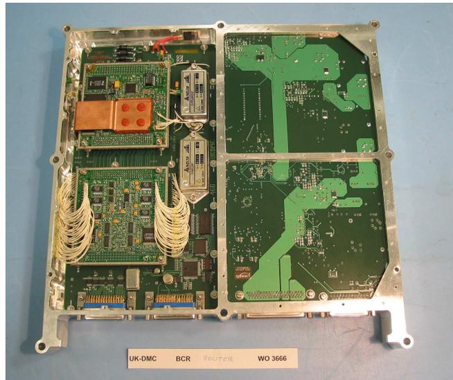
At back left: router card with heatsink brace in place. At front left: serial card is connected to payloads via half-width motherboard under cards.
