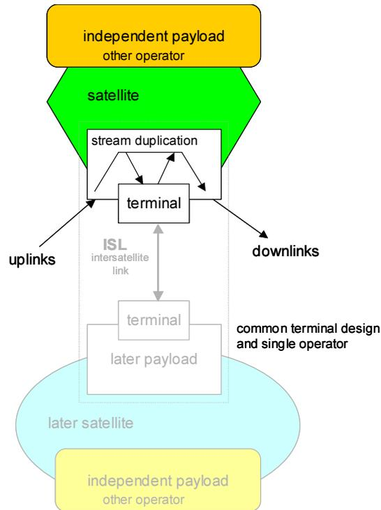
**Figure 1: first satellite payload capable of streaming uplinked traffic to/from ISL**
