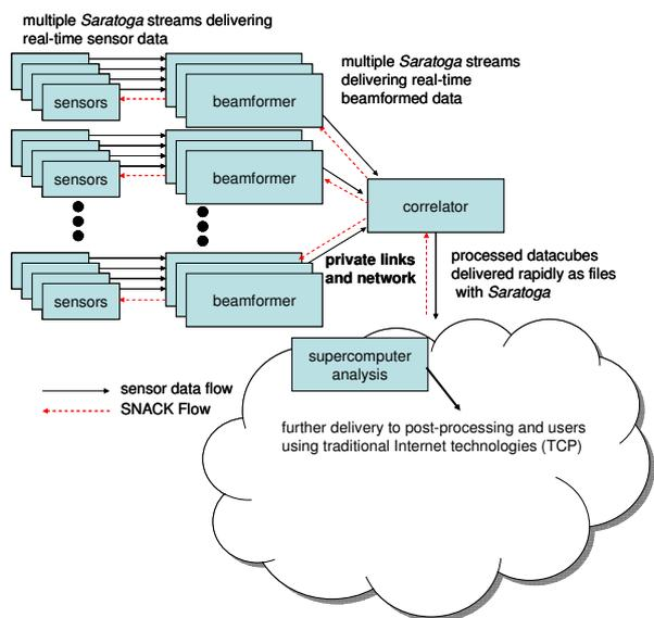
**Figure 3 – proposed uses of *Saratoga* in radio astronomy**
