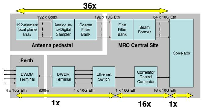
Figure 5 – Data Flow & Processes in ASKAP
