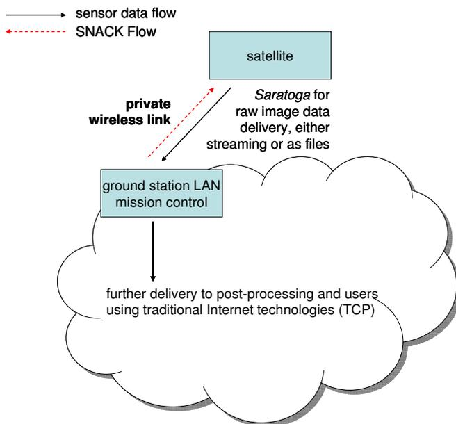
Figure 1 – Use of *Saratoga* for remote-sensing satellites
