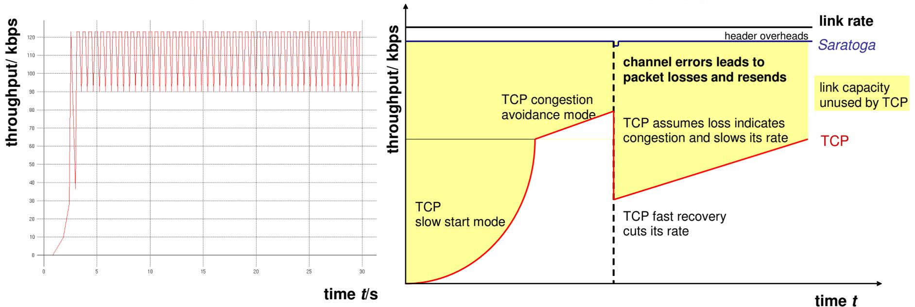
A single TCP flow can't fill a link – reaches capacity, then backs off.
