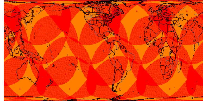
Lower elevation angle gives dual coverage (but not double surface coverage)
