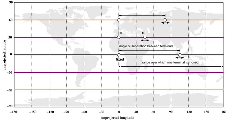
Teledesic *with* and *without* cross-seam links; every line shows a 24-hour simulation at a given latitude separation between terminals. Smaller delays and delay variation *with* cross-seam links. Note difference at 0° separation.
