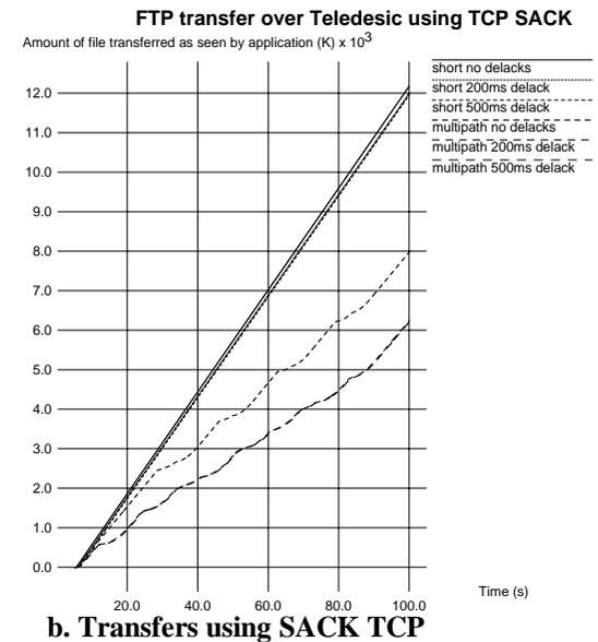
Progress of FTP transfer between terminals at Quito and Tokyo using *Teledesic* delayed acks degrading file transfer over multiple LEO paths
