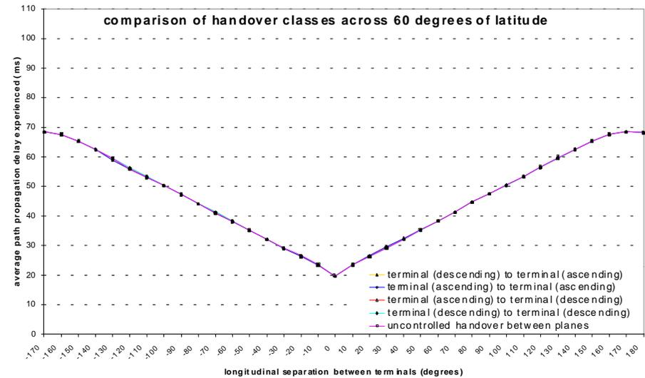
Uncontrolled handover falls between two limits. At limits of coverage (60° latitude) effect vanishes.
