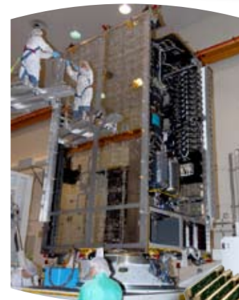
IntelSat 14 (IS-14) being built by Space Systems / Loral
