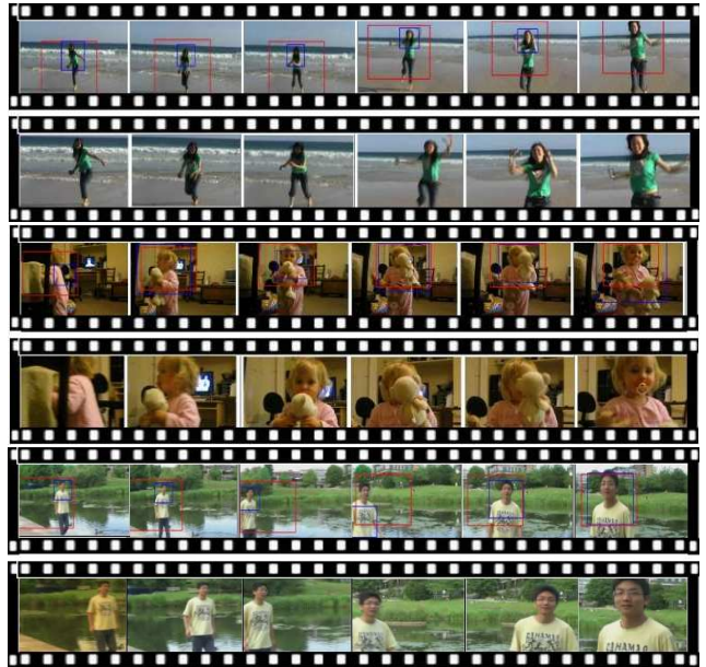
Figure 8: Final edited clip results from footage V3 – V5. Upper strip: Blue box indicates interest detection, red box indicates cropping window. Lower strip: Footage is rendered from within the red window to output the final clip.
