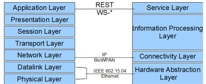
Fig 2: OSI model and mapping to different layers
