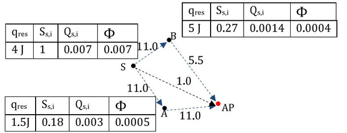
Fig. 3. Illustration of the NetCoop cooperation strategy. Here, relay B is chosen instead of A as the latter has low residual energy.
