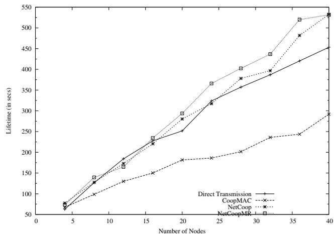
Fig. 5. Network Lifetime of Multi-Relay cooperation compared to the three other schemes.
