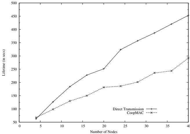
Fig. 1. Network lifetime of CoopMAC when compared to that of direct transmission.
