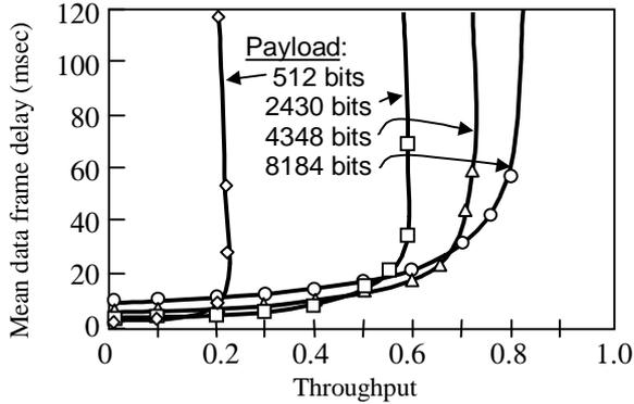
Figure 5: The delay performance of the IEEE 802.11 MAC protocol with the four-way handshaking access method
