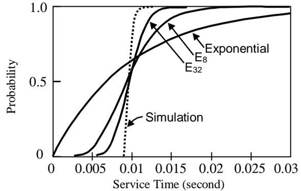
Figure 4: The CDFs of an exponential, Erlang random variables and the service time of the IEEE 802.11 MAC protocol for  $k=20$  and payload=8184 bits
