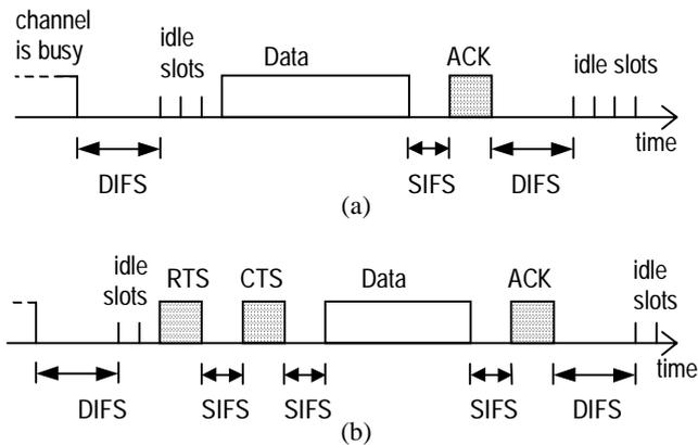
Figure 1: The IEEE 802.11 access methods: (a) Basic access method. (b) Four-way handshaking access method
