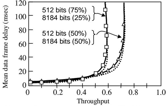
Figure 7: The delay performance of the IEEE 802.11 MAC protocol for dual fixed data frame size
