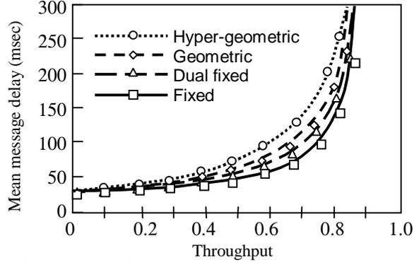
Figure 8: The delay performance of the IEEE 802.11 MAC protocol for trains of data frames
