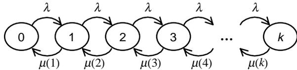
Figure 3: The state dependent service rates M/M/1/k queue for the analysis of a MAC protocol
