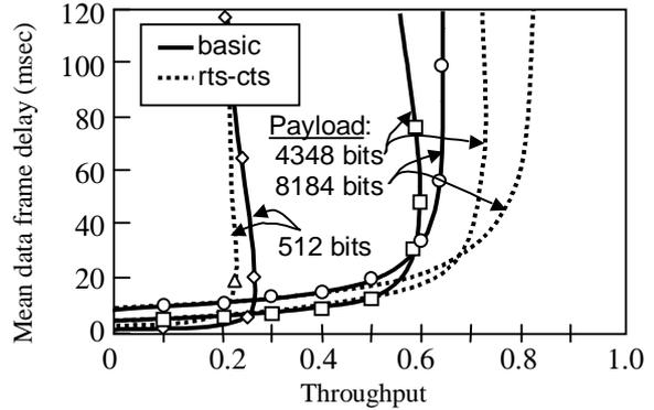
Figure 6: The delay performance of the IEEE 802.11 MAC protocol with the basic access method
