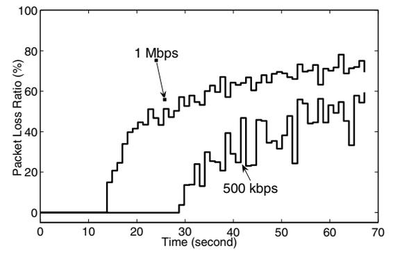
Fig. 7. Packet loss ratio for EDCA.
