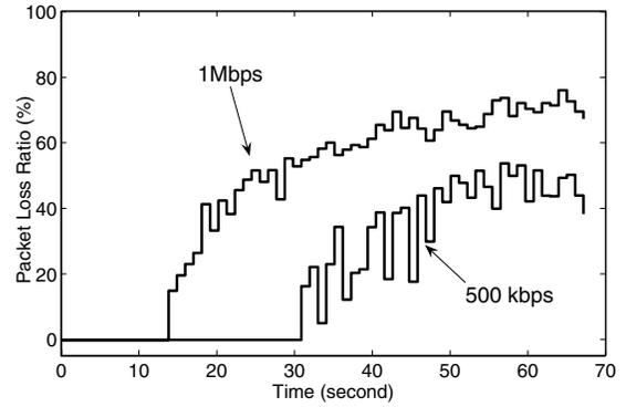
Fig. 6. Packet loss ratio for DCF.
