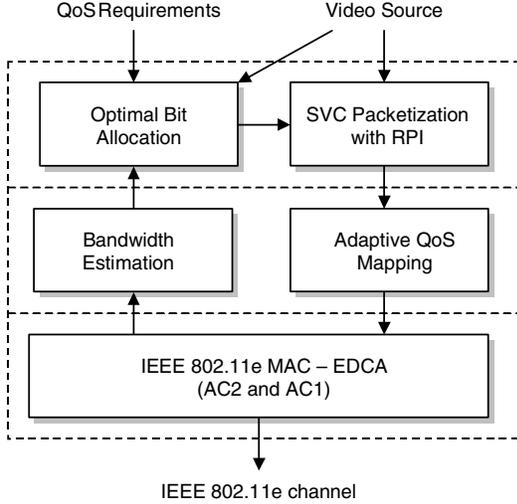
Fig. 1. Block diagram of the proposed cross-layer QoS design.
