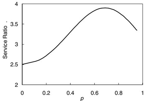
Fig. 2. The ratio of the throughput of AC2 to that of AC1 in an EDCA node under various network load conditions.
