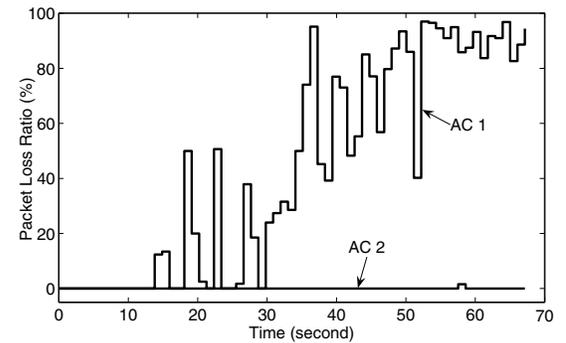
Fig. 8. Packet loss ratio for our cross-layer design.
