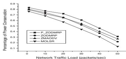
Fig. 15. Average power conservation Vs. network traffic load
