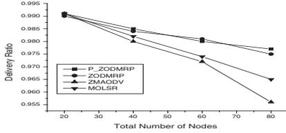
Fig. 8. Delivery ratio Vs. node vicinity density
