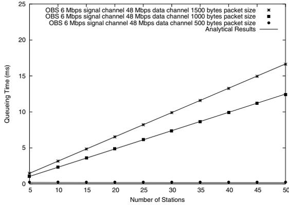
Fig. 5. Average queuing delay of OBS scheme.
