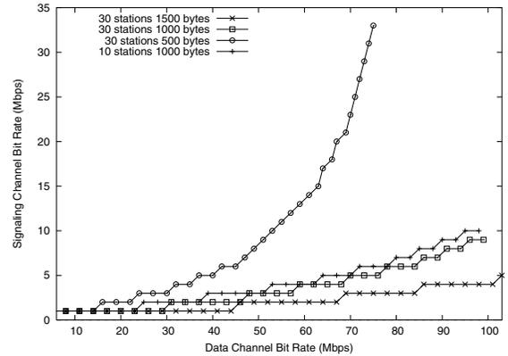
Fig. 7. Minimum signaling channel data rate required to achieve full utilization on the data channel for a total data rate up to 108 Mbps.
