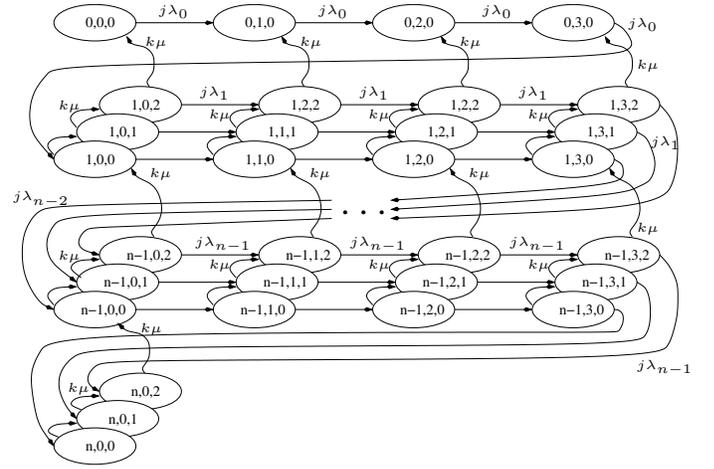
Fig. 2. Markov chain model of a  $E_4/E_3/1/n$  queue.
