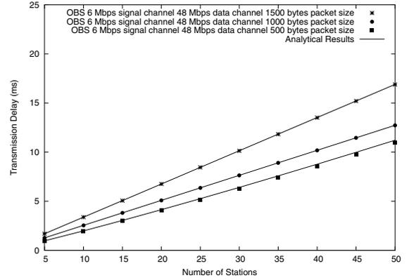
Fig. 4. Average transmission delay of OBS scheme.
