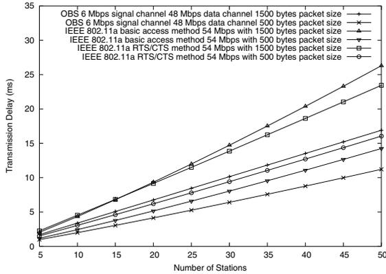
Fig. 6. Average transmission delay of OBS scheme compared with the IEEE 802.11a.
