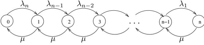
Fig. 7. State transition diagram of the birth-death process representing the state of the data channel's queue.
