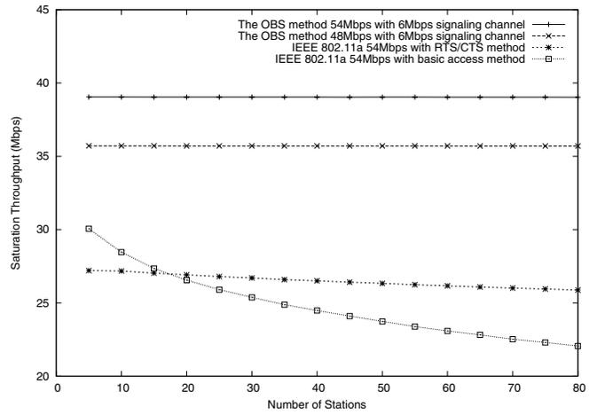
Fig. 4. Saturation throughput of the high speed channel.
