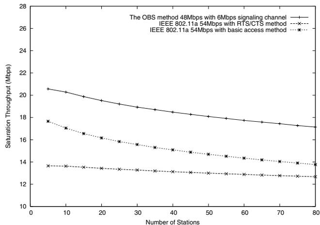
Fig. 8. Saturation throughput of the high speed channel with 500 bytes packet size.
