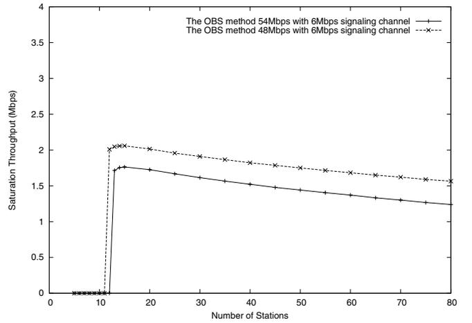
Fig. 5. Saturation throughput of the low speed (signaling) channel.
