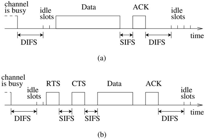
Fig. 1. IEEE 802.11 DCF: (a) Basic access method. (b) Four-way handshaking method.
