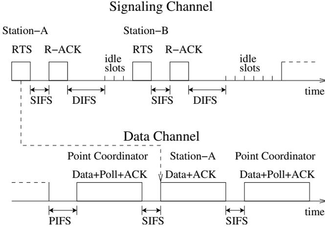
Fig. 3. The OBS scheme using out-of-band signaling.
