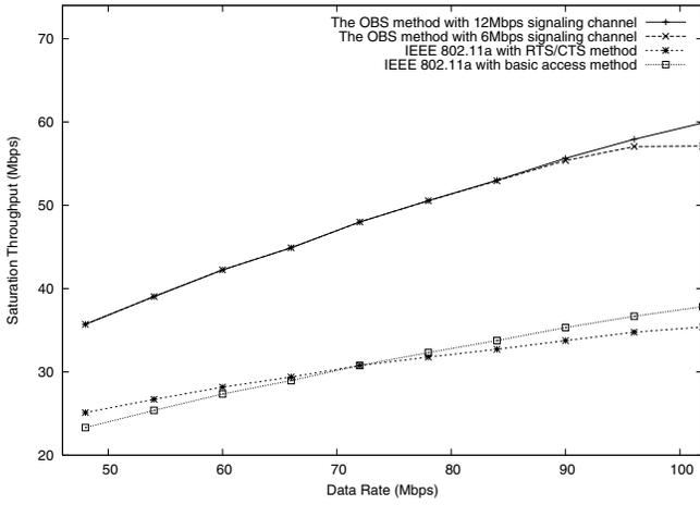
Fig. 6. Saturation throughput versus data rate with 30 stations.
