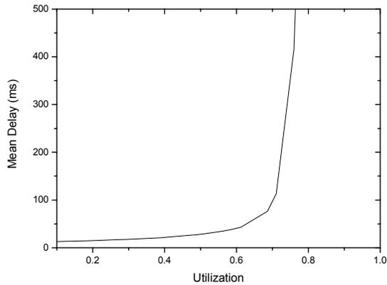
Fig. 6. Mean delay versus utilization for OBS bursts
