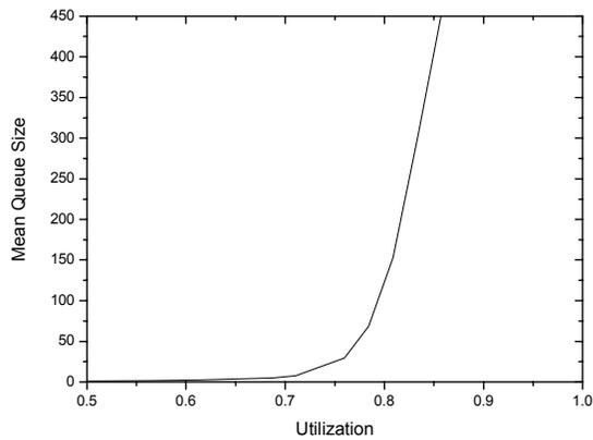
Fig. 7. Mean queue size versus utilization
