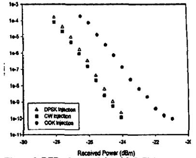
Figure 5. BER of re-modulated 2.5-Gb/s upstream data stream for CW, DPSK and OOK injection measured at central office.
