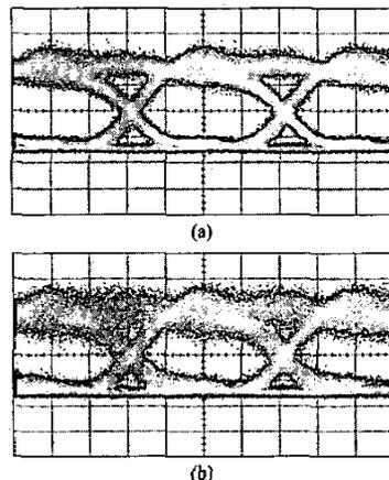
Figure 4. Eye diagram of re-modulated 2.5-Gb/s upstream data with (a) CW-injection and (b) DPSK-injection measured at central office.
