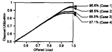
Fig. 3. Channel utilization versus offered load for FULL-RCMA
