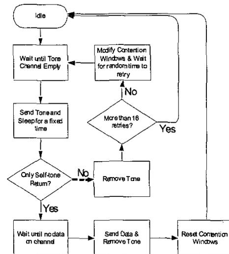
Fig. 1 Algorithm of the Collision Avoidance Protocol Pilot Tone-based carrier sense mechanism
