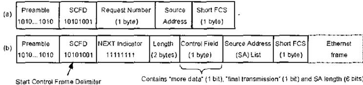
Fig. 2. The frame format (a) FULL-RCMA request frame (b) FULL-RCMA NEXT frame
