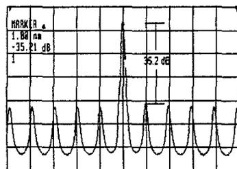
Figure 3. Output optical spectra of the injection-locked signal by downstream wavelength (1546.73nm) with an SMSR of 35.2dB
