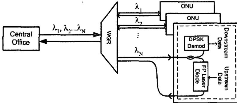
Figure 1. WDM PON using DPSK as downstream modulation format and upstream data remodulation using injection locked FP laser.
