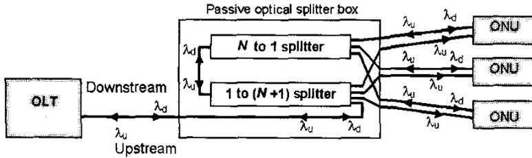
Fig. 1. Network Architecture of FULL-RCMA
