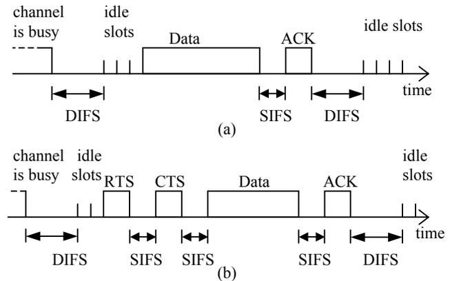
Fig. 1. IEEE 802.11 access methods: (a) Basic access method. (b) Four-way handshaking access method.
