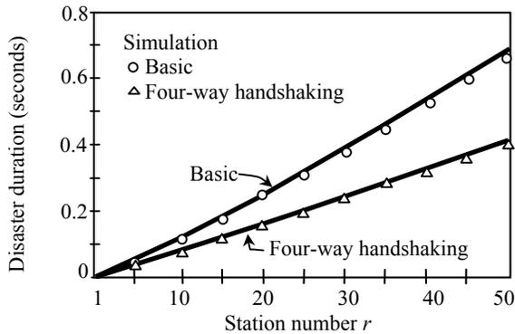
Fig. 6. The disaster duration of IEEE 802.11 for  $CW_{min}=8$  and  $CW_{max}=256$
