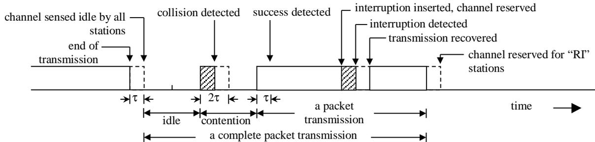
Fig. 1. A snapshot of the broadcast channel of CSMA/RI
