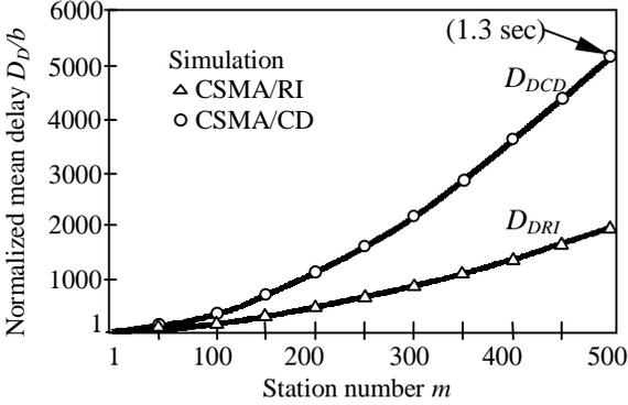
Fig. 8. The normalized mean delay in the disaster scenario for  $b=5$
