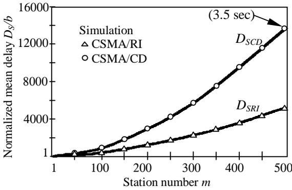
Fig. 4. The normalized mean delay in the saturation scenario for  $b=5$
