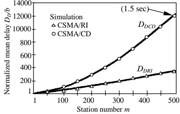
Fig. 9. The normalized mean delay in the disaster scenario for  $b=25$
