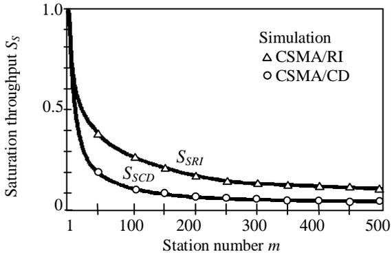
Fig. 2. The saturation throughput for  $b=5$
