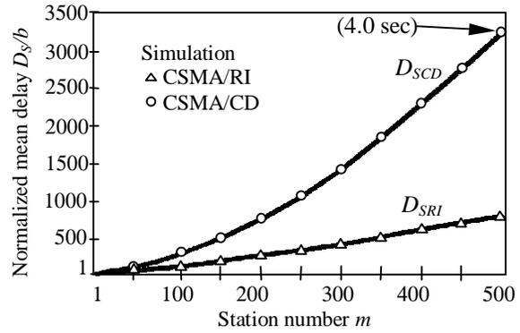
Fig. 5. The normalized mean delay in the saturation scenario for  $b=25$
