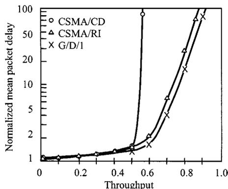
Fig. 13. CSMA/CD and CSMA/RI: normalized mean packet delay versus throughput for  $b = 50$  and traffic burstiness = 0.5.
