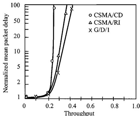
Fig. 15. CSMA/CD and CSMA/RI: normalized mean packet delay versus throughput for  $b = 10$  and traffic burstiness = 0.2.
