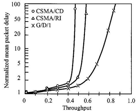
Fig. 12. CSMA/CD and CSMA/RI: normalized mean packet delay versus throughput for  $b = 50$  and traffic burstiness = 0.2.
