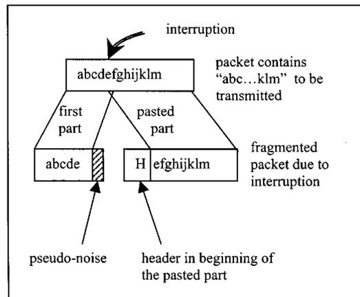
Fig. 2. The fragmented packet presented to the receiver.
