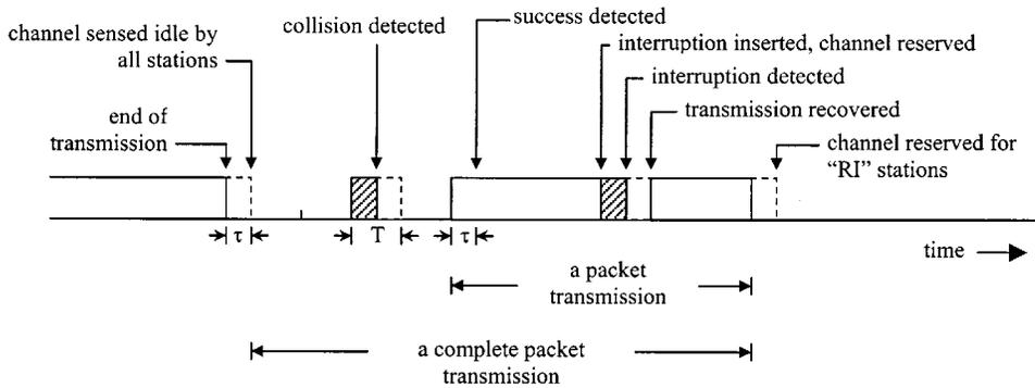
Fig. 1. A snapshot of the broadcast channel of CSMA/RI.
