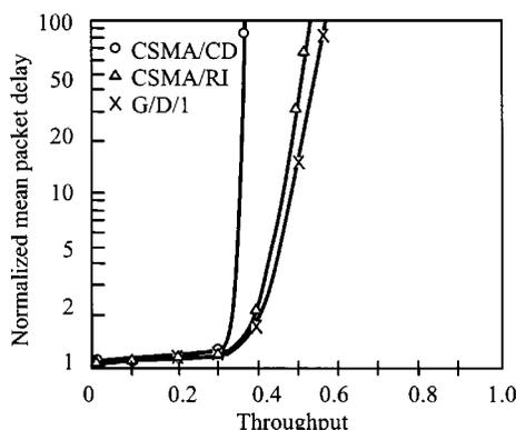
Fig. 14. CSMA/CD and CSMA/RI: normalized mean packet delay versus throughput for  $b = 50$  and traffic burstiness = 0.8.
