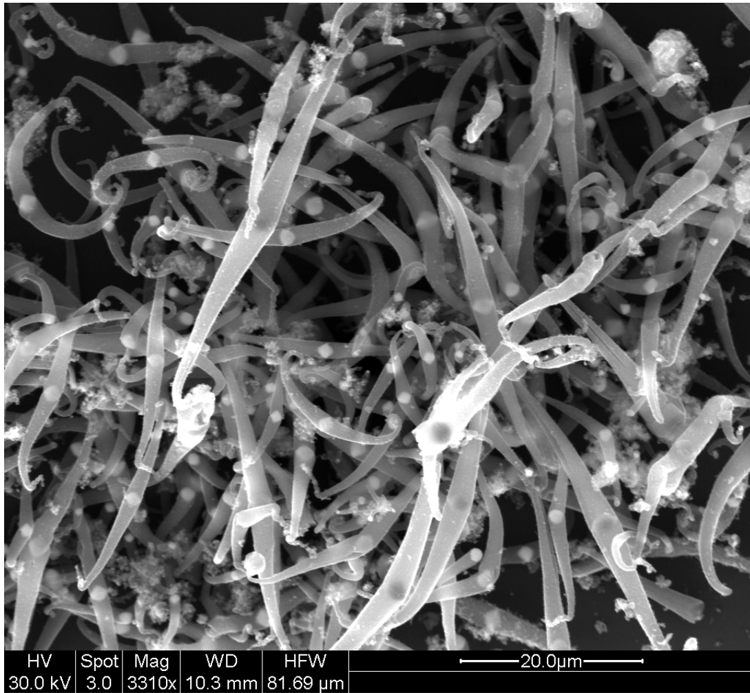
Figure S1: Large-scale scanning electron micrograph, showing the micro-cones produced in high yield at 6.1 MPa.
